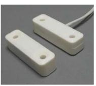
IO 102-16/2 security magnetically contact detector is designed for locking doorways and windows, arranging "trapping" medium as well as locking other elements of buildings with an alarm signal raised to a control panel, concentrator or central surveillance system by opening reed switch contacts.
