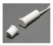
IO 102-15/2 security magnetically contact detector is designed for locking doorways and windows, arranging "trapping" medium as well as locking other elements of buildings with an alarm signal raised to a control panel, concentrator or central surveillance system by opening reed switch contacts.
