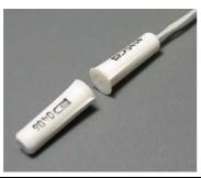
IO 102-15/1 security magnetically contact detector is designed for locking doorways and windows, arranging "trapping" medium as well as locking other elements of buildings with an alarm signal raised to a control panel, concentrator or central surveillance system by opening reed switch contacts.
